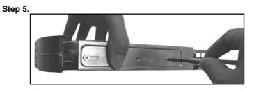
Secure the HDD and the Inner Cradle with four retaining screws (two on each side).
